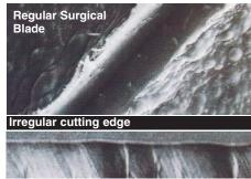
A regular surgical blade leaves a ragged edge as indicated by a lack of uniform smoothness when cutting the polystyrene.
