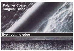
Smooth, clean cut is illustrated by cutting through 10 mm polystyrene (magnified 750 times). Our precision grinding technology coupled with our advanced polymer coating process, provides a significantly improved cutting edge.
